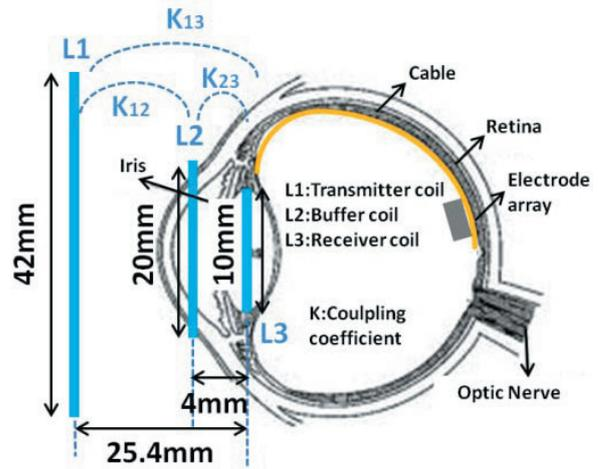
Figure 4. The 3-coil scheme for inductive power transfer.
