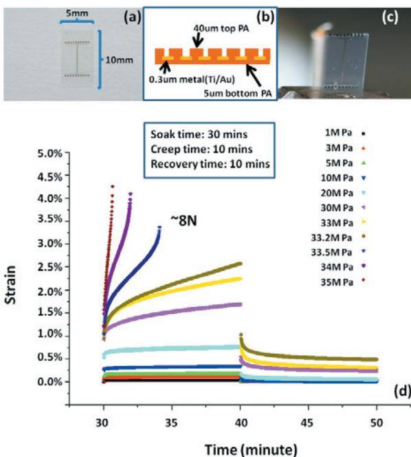
Figure 10. (a) Parylene flex test sample. (b) Cross-section of the tested sample. (c) Broken sample caused by over-stress. (d) Creep test at body temperature of 37°C.
