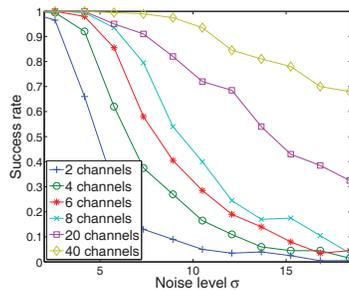
**Fig. 3:** Same setup as Fig. 2. The overall data output rate is fixed, and the number of channels is varied (as the number of channels increases, the sampling rate of each channel decreases). Designs with more channels are more robust to noise.
