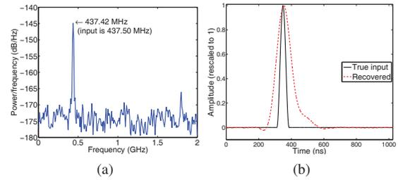
**Fig. 5:** (a) Recovery of a tone with amplitude  $400\mu V_{pp}$ , which is  $-53.98$ dB below the full-scale amplitude. The frequency estimation is accurate to within 0.08MHz. 512ns worth of samples were used. (b) Recovery of a 75ns pulse. Frequency estimation accurate to 1.02MHz.
