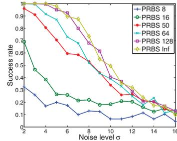
Fig. 2: Success rate of frequency estimation across noise, for various PRBS repetition lengths, via simulation. The noise level is unphysical, and for comparison purposes only. A PRBS of length 128 or higher is most robust to noise. A “success” is defined as estimation error of less than 5MHz (each data point is the outcome of 200 independent trials)
